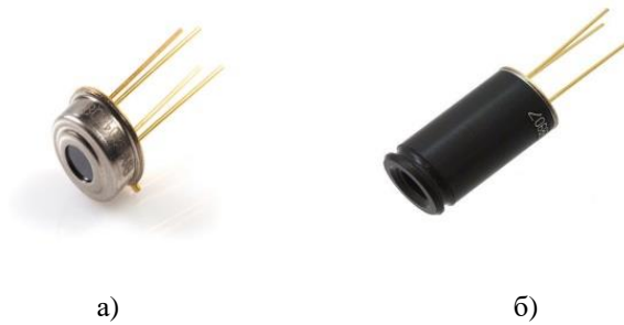
a) b) Figure 3 – Exterior of the MLX90614 meter: a - without refraction filter, b - with refraction filter
